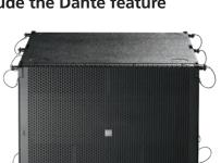
**MUSE218SND/218SN** is a direct radiation ground subwoofer, it has 2 B&C **460mm (18")** long-range woofers and 4000W class D amplification capable of 148.5dB SPL. The subwoofer serves as the basis for ground-stack configurations and is equipped with a preset for cardioid configuration.
